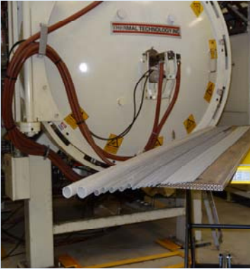
AMS Vacuum/Hydrogen Sintering Furnace with Metallic Membranes
